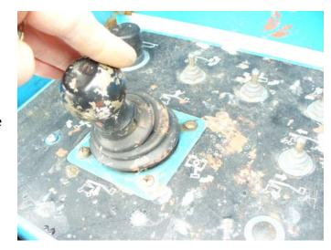
When the desired boom creep speed has been achieved move the drive enable switch to the left or right once and release it while maintaining the joystick position.
